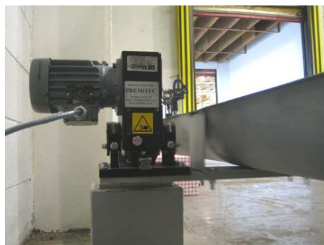
Floor mounted Vibratory Motor & Gearbox.
