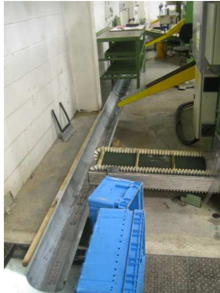
14 Meter tray taking scrap away behind four presses.
