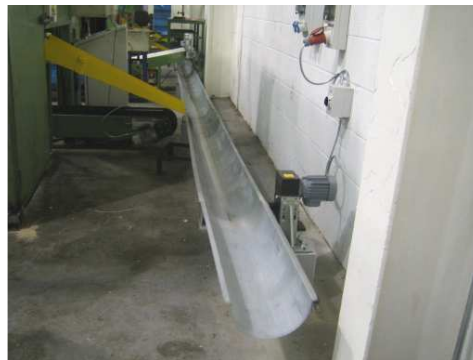
Gearbox attached to the tray.
