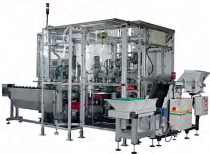
ENSAMBLAJE DE RÓTULAS ASSEMBLY OF BALL JOINTS KUGELGELENKMONTAGE
