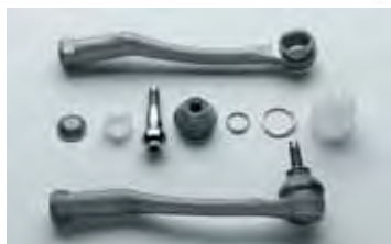
ENSAMBLAJE DE RÓTULAS ASSEMBLY OF BALL JOINTS KUGELGELENKMONTAGE
